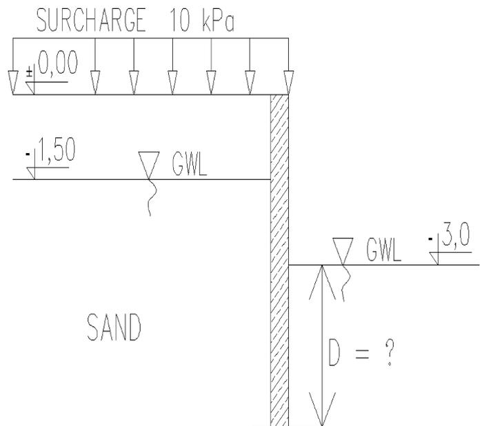
Figure 1. First example case - geometry and soil conditions.
