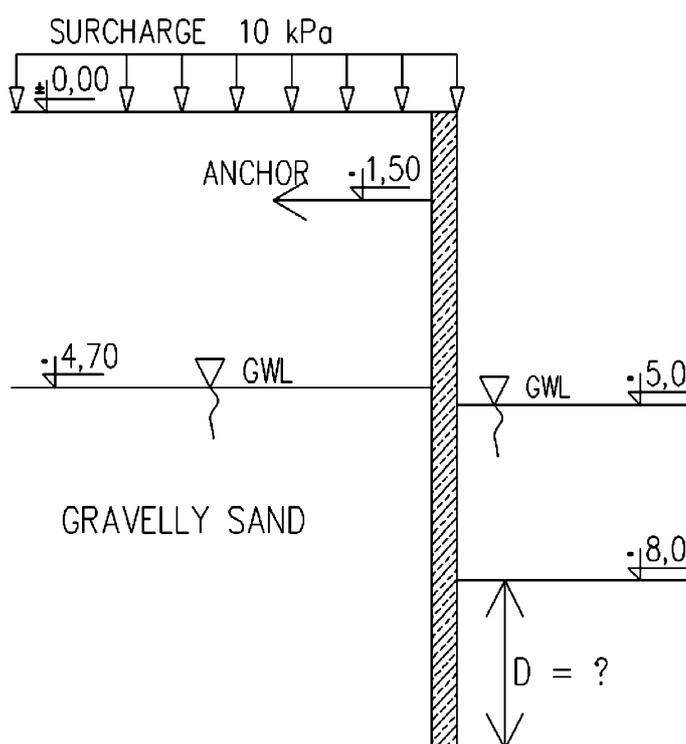
Figure 2. Second example case – anchored diaphragm wall.
