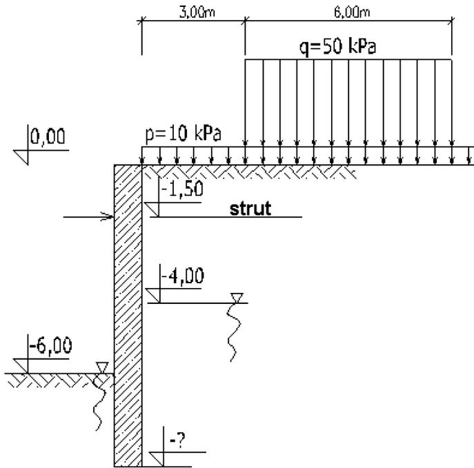
Figure 3. Third example case – strutted diaphragm wall.
