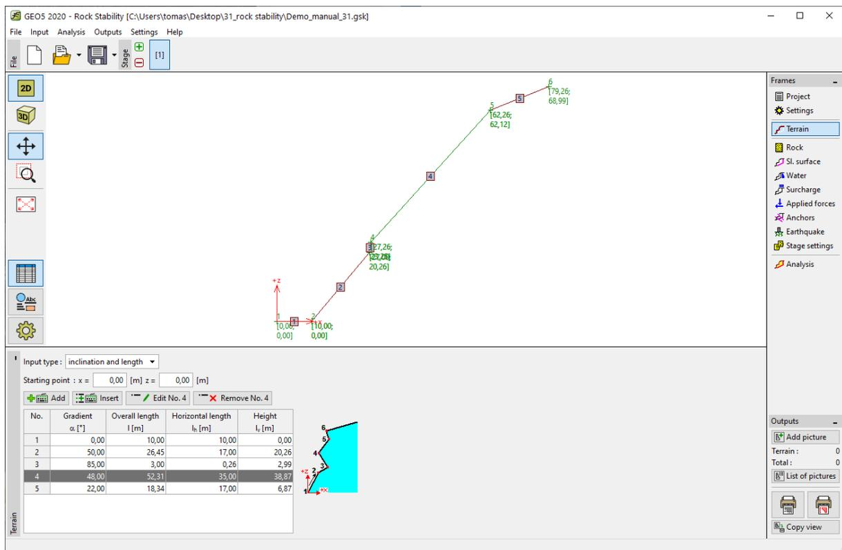
*Cross-section setting of line segments in "Terrain" frame.*
