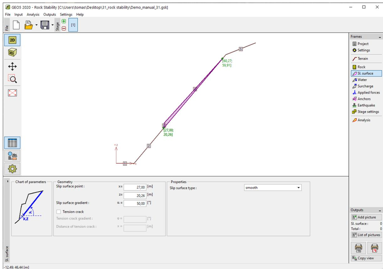
*Shear failure settings in the “Slip Surface” frame*
